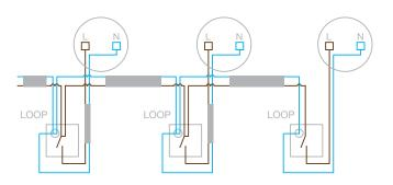
As can be seen from the diagram the neutrals are looped through the switches with a single line and neutral to each light fitting.
