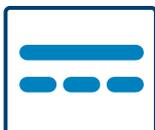
RCD can detect & respond the same as Type F + **smooth DC residual current.**
