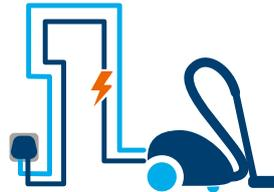
Arc fault detection devices (AFDD) use microprocessors to identify characteristic current flow and voltage curves that indicate an arc fault and automatically trip the affected circuit.
