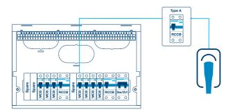
This design does have an individual RCD supplying the car charger.
