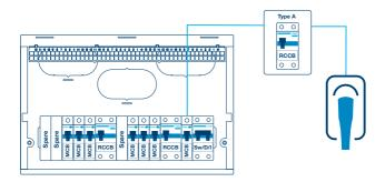
If the cable does require RCD protection then a DP RCBO, 30 mA Type A could be selected as the protective device as in this example. An additional RCD closer to the car charger will not be required.
