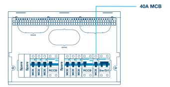
ii) RCD is required to supply car charger that has RDC-DD of 6mA. Or cable requires additional protection by RCD. Either of these can be satisfied with Double Pole Type A RCBO within consumer unit.
