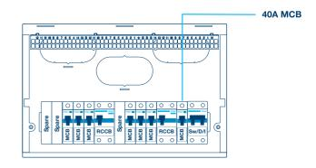
ii) RCD is required to supply car charger that has RDC-DD of 6mA. Or cable requires additional protection by RCD. Either of these can be satisfied with Double Pole Type A RCBO within consumer unit. For more information, please contact our Technical Helpline.
