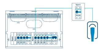
In this example the MCB is giving overcurrent protection (does not have to switch neutral) and the RCCB Type A has been installed close to the car charger.
