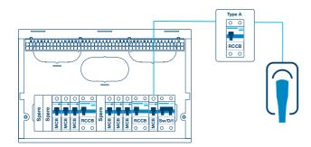
If the Consumer Unit is a newer version that already contains a Type A RCCB then there is no concern as the secondary RCCB closer to the car charger will not be required as shown below.
