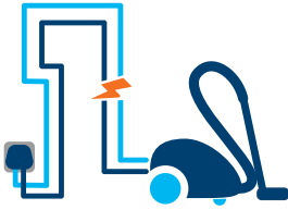
Parallel Arc Fault
